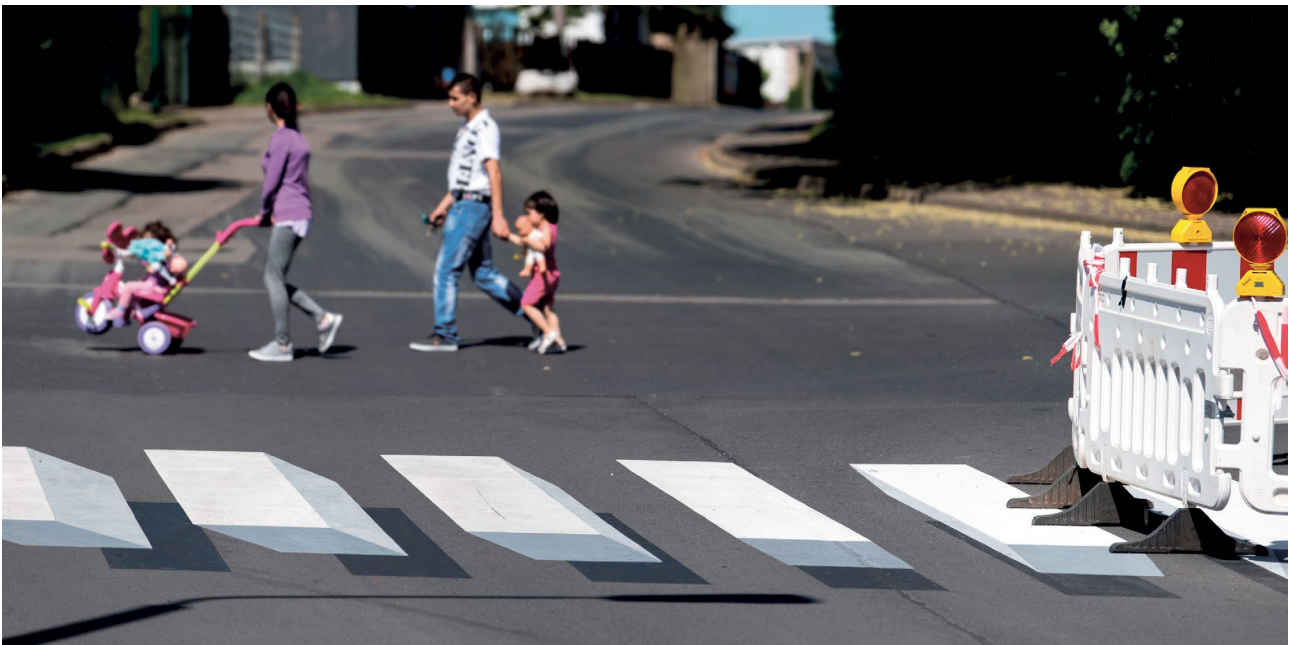
Figure 4: Optical illusion which might fool a camera-based perception system
